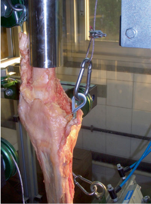
Fig. 21.5 The same knee with the meniscus already repaired and the osteotomy fixed, mounted in a gait simulator to test the repair (Courtesy of X. Pelfort M.D.)
