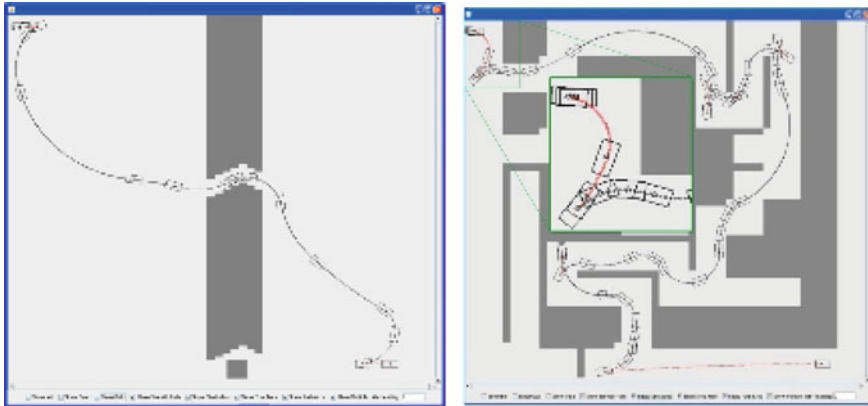
Fig. 5 PRM-AS path solution in the “corridor (maze)” environment. The magnified area ( green box ) shows the maneuver ( red curved line ) undertaken to exit the tight space ( bottom right of green box ) while positioning the vehicle for forward movement (Balakirsky and Dimitrov 2010). The maneuver ( red curved line ) also indicates the vehicle moving in reverse
