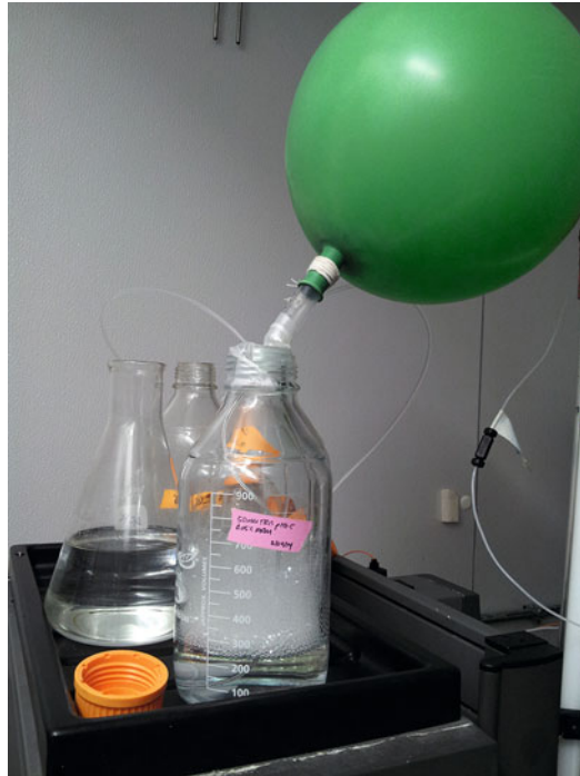
Fig. 3 Example of purification buffer setup. Balloons filled with argon are secured to a bottle containing degassed buffer using a syringe and parafilm. Argon slowly bubbles through the solution via tubing that attaches to the syringe and runs to the bottom of the bottle
