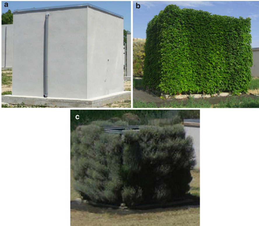
Fig. 23 Studied cubicles in the experimental set-up (a) Reference; (b) green wall A; (c) green wall B [40]
