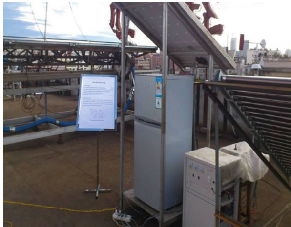
Fig. 18 Working diagram of solar photovoltaic refrigerator
