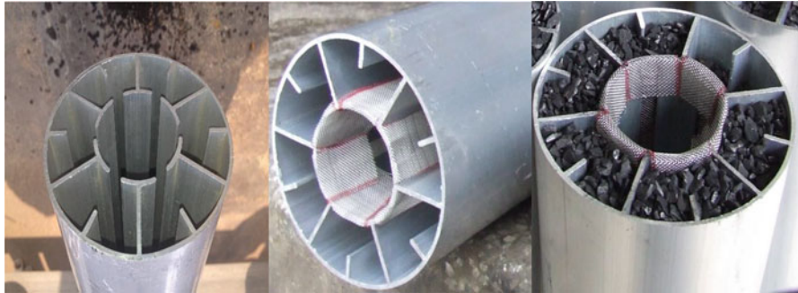
Fig. 4 Configuration of the finned-tube adsorption casing
