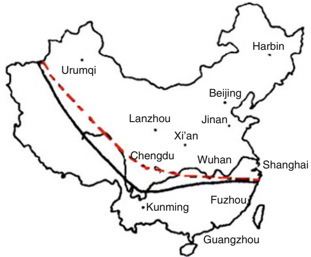
Fig. 37 Suitable applied areas of WLHPS when electric boiler used in China (North area of the dash line) [70]
