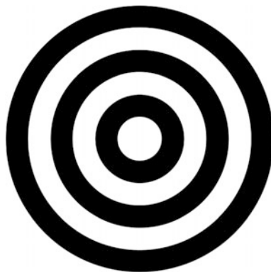
Fig. 7 A typical Bessel beam profile. The white regions (indicating laser beam) show negligible diffraction over the working range of a microscope, meaning they can be used over longer distances than a normal Gaussian trap
