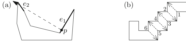
Fig. 1. (a) Normal ray \text{ray}_{e_1}(p) and a pair of conflicting edges e_1, e_2 . (b) The heuristic in [19] splits a non-greedy region by a bisector at a maximum reflex angle. If the splits are chosen in order of their index, seven regions are created, although two is minimum (split only at 6).
