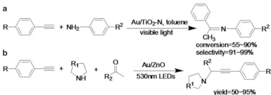
Scheme 8.13 Photocatalytic C–N coupling reactions between alkynes with amines (Reprinted with permission [33]. Copyright 2014 Royal Society of Chemistry)
