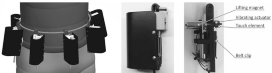
Fig. 2 Mounted actuator units as 3D-CAD model ( left ), single unit with cover ( middle ) and described components ( right )
