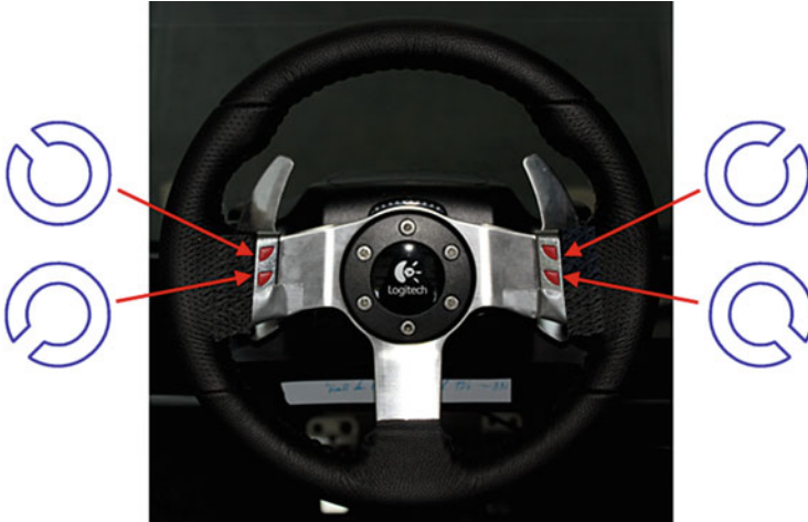
Fig. 5 Steering wheel with the button corresponding to the orientation of the gap of the Landolt ring
