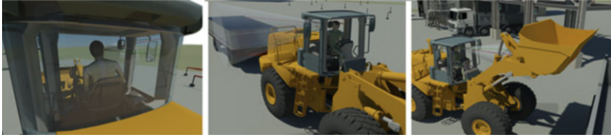
Fig. 4 Holistic virtual copy of work tasks, including body and eye movements of test persons attached to their individual digital representatives, combined with the movements of the wheel loader as virtually operated by the test persons in the interactive simulation [4]
