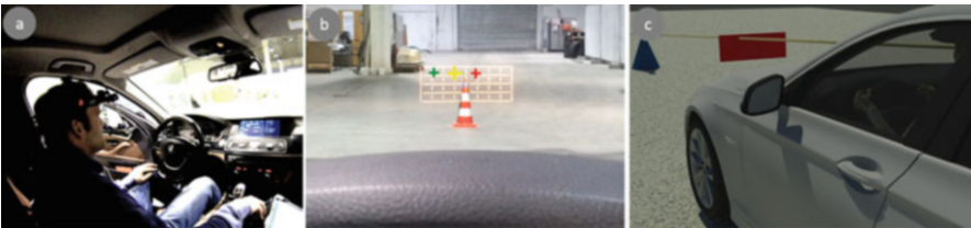
Fig. 10 Differentiation of fixated objects by an eyetracked test person (a), if these are aligned one behind the other (b) within an animated scenario in the 3D-modelling environment 3DS max (c)
