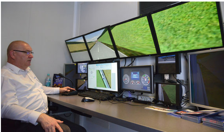
Fig. 3 Trainer cabin of the mobile truck simulator (SiFaT Road Safety GmbH)
