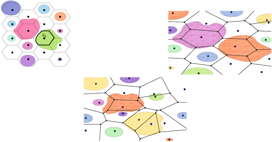
Fig. 1. The overlay of an SINR diagram of a nonuniform wireless network on the corresponding Voronoi diagram. (a) Hexagonal Voronoi cells; the intersection between the reception region of station s_0 and the Voronoi cell around it is highlighted in bold. (b) Slight random perturbation to a hexagonal network. (c) Random positions.
