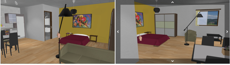
Fig. 3. Three-degrees of freedom interface. At left with a mouse input device: the cursor (shown as a hand) is centered, the mouse movement is mapped to the yaw and pitch angles, and selection is always done at the center of the window where the cursor is fixed. At right with single-touch screen, the frame is used for camera orientation, and the cursor is free for selection at any point of the window. Users do not need to change the orientation to select an object visible in the current frame.
