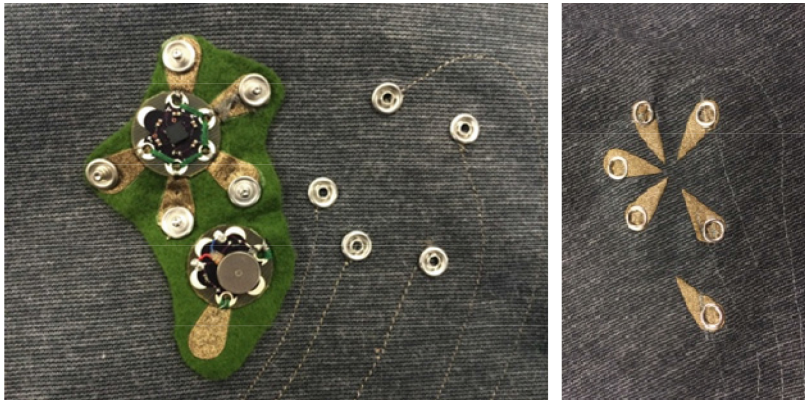
Fig. 5. Conductive fabric pattern for Accelerometer.
