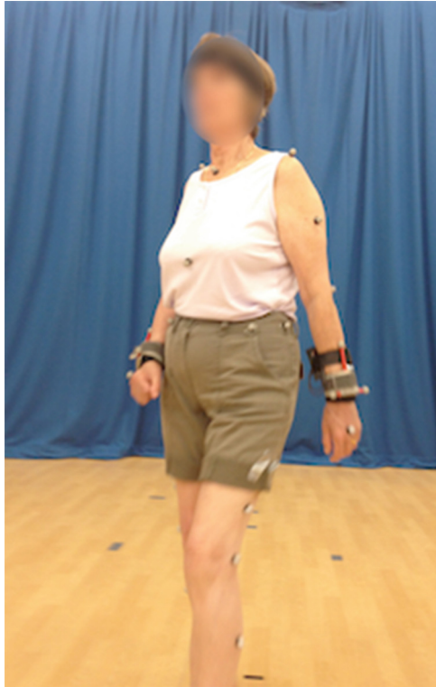
Fig. 3. Tactile cued walking of a stroke survivor. As well as wearing a haptic bracelet on the paretic (right arm), the participant is wearing optical markers on the body for motion tracking.
