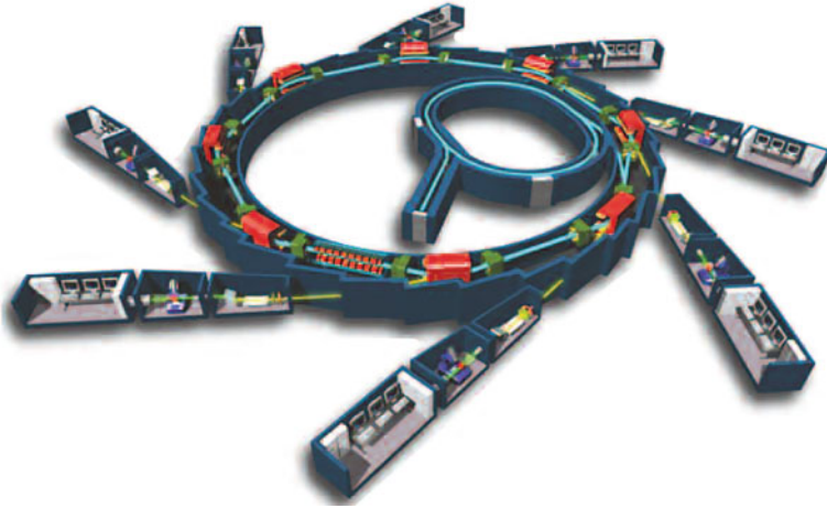
Fig. 8.2 Schematic drawing of a third-generation synchrotron machine (SOLEIL synchrotron, France)
