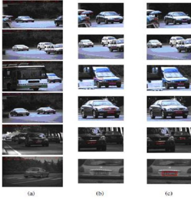
Fig. 5. Comparison results:column(a) images processed by color algorithm alone,column(b) magnified portion of images showed in column(a),column(c) images processed by adaboost algorithm combined with color differential feature
