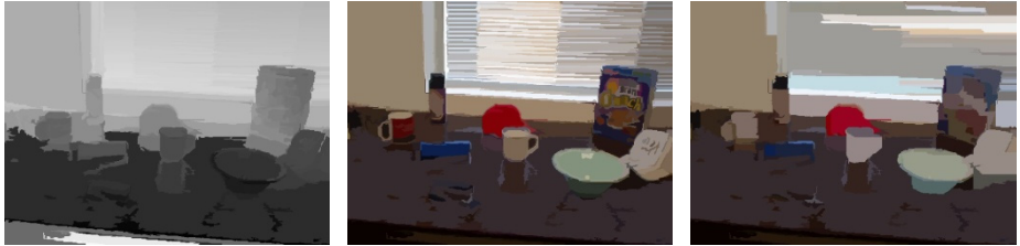
Fig. 2. Graph-cut based Superpixel segmentation on three type of data (top-left: raw RGB, top-right: raw depth; bottom-left: segmentation on depth, bottom-middle: segmentation on Lab, bottom-right: segmentation on Depth + Lab)
