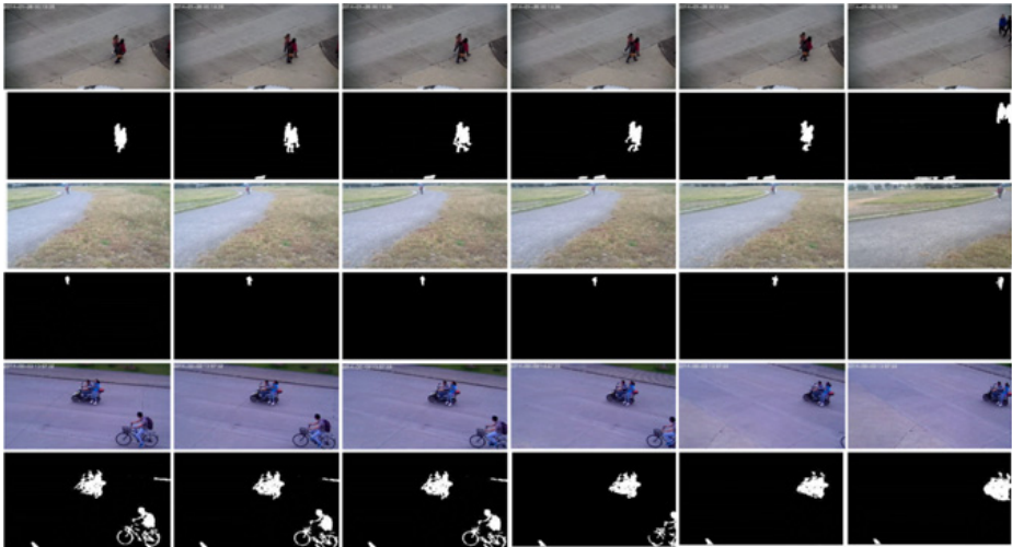
Fig. 6. The detection results of our proposed algorithm on 3 videos in every 5 frames. The 3 odd rows are the frames from 3 test videos respectively and the other 3 even rows are the corresponding detection results by our proposed method.
