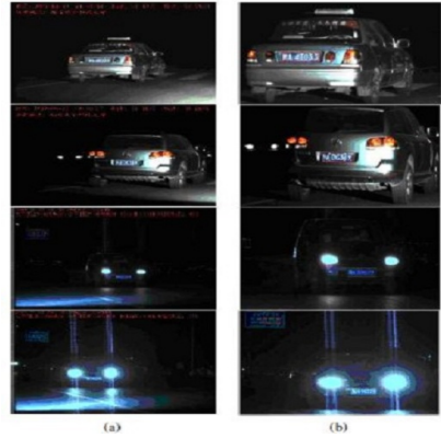
Fig. 6. Experiment results:column(a) original color images gained at night,column(b) images processed by adaboost algorithm combined with color differential model
