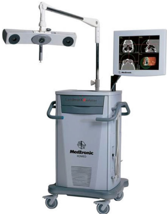
Fig. 20.3 Optical-based image-guidance system. Infrared camera is located within the horizontal bar above the video monitor
