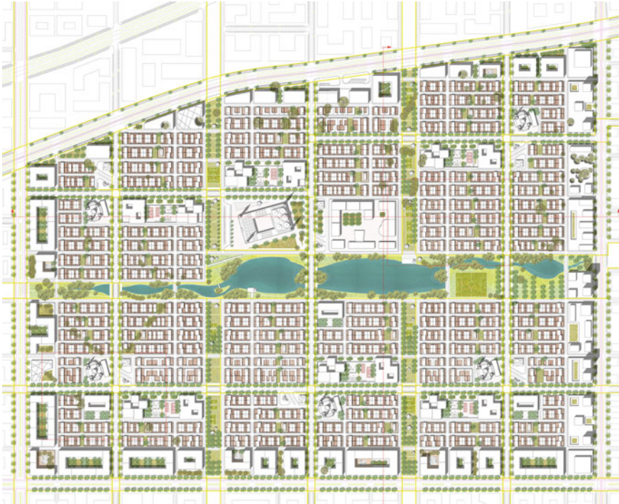
Fig. 21.15 Local storm water management through green networks and road surface drainage in a Jumma City district for up to 40,000 inhabitants. Image by COBE Berlin
