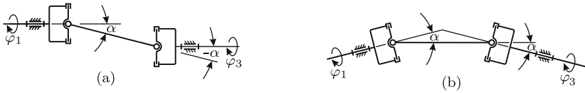
Fig. 13.6 The two possible couplings of coplanar shafts 1, 2, 3 by two Hooke's joints resulting in \dot{\varphi}_3 \equiv \dot{\varphi}_1
