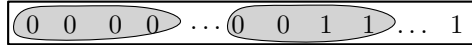
Fig. 2. Consider one row that is being converted to column-major layout. The elements that will be put in the same column are bundled together. It is easily seen that each row will create at most one dirty column.
