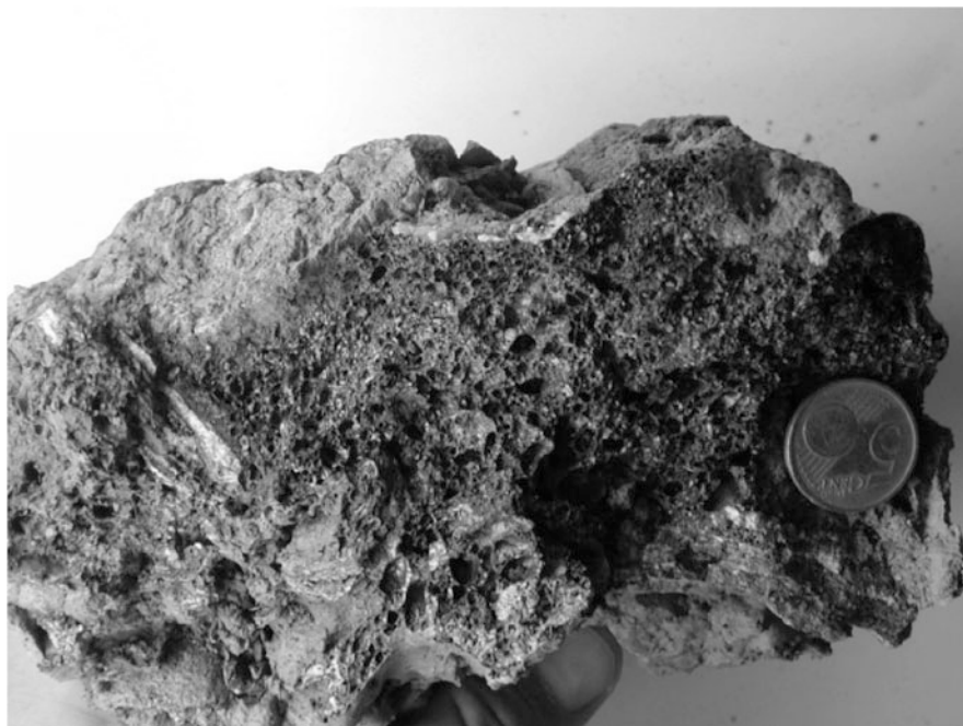
Fig. 2 Hand specimen of s slag sample from the Goldbichl site. The slag is characterized by a multitude of vesicles indicating a high amount of sheet silicates in the protolith rock. Relict patches of quartzphyllite can still be seen on the left side
