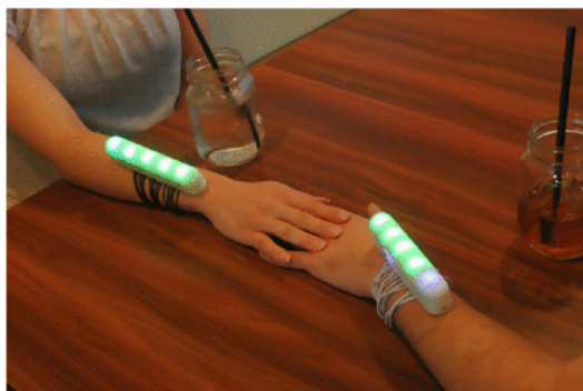
Fig. 8. An olfactory-based interactive wearable application to emit a delicate fragrance, called Light Perfume, was developed by Choi et al. [21] from Keio University.
