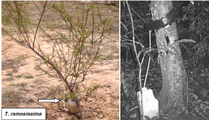
Fig. 26 Stemflow collector consisting of plastic tubing and a collection bottle. Left figure for shrubs (Li et al. 2008) and right figure for trees (Germer et al. 2010)
