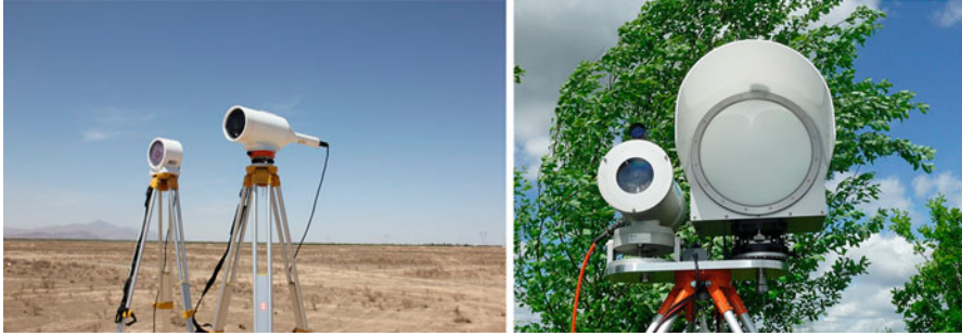
Fig. 5 Scintillometer (LAS (BLS450, Scintec) and MWS; the picture on the right is from the RPG manual)
