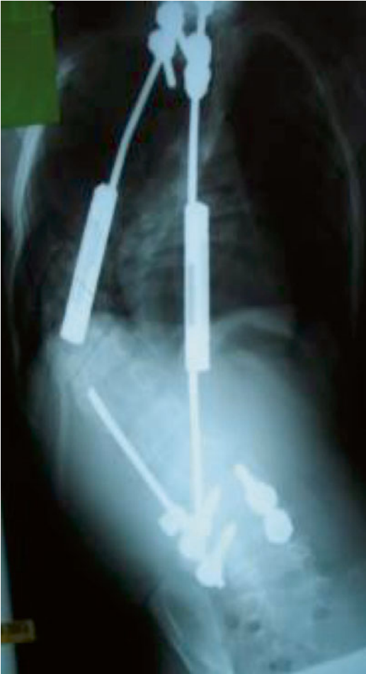
Fig. 3.5 Clinical example of a stress concentration. When a device changes abruptly from a smaller diameter to a larger diameter, a stress concentration is created. Here it is shown that the abrupt transition of the coupling point to the rod caused the device to fail. A rod of larger diameter may have minimized the potential for failure by reducing the stress concentration between the coupling and the rod
