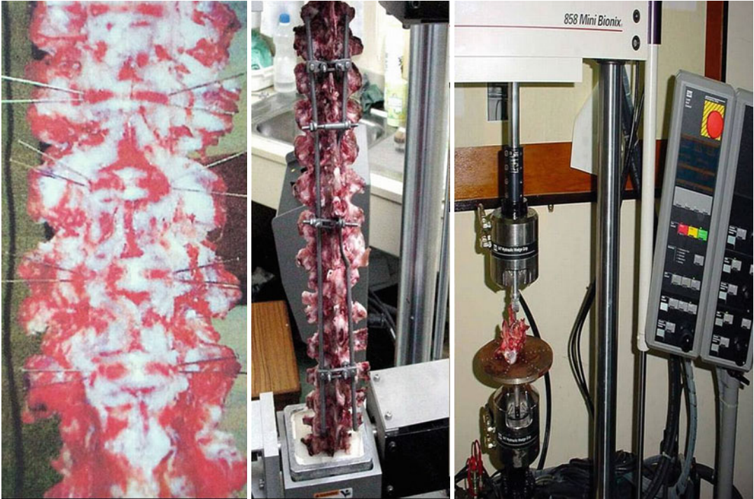
Fig. 49.3 Biomechanical test using porcine spine model
