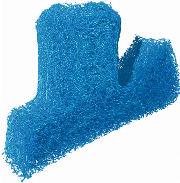
Fig. 5 Visualization of a glass fiber-reinforced polymer, imaged using X-ray computed tomography (visualization: H. Riedel, Fraunhofer ITWM, department “Image processing”)
