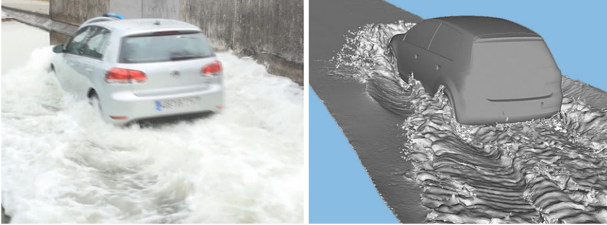
Fig. 2 A further example for the application of the FPM method: a car driving through water; experiment and associated FPM simulation (photo and simulation: Volkswagen, Inc., as part of a cooperative project with the Fraunhofer ITWM)
