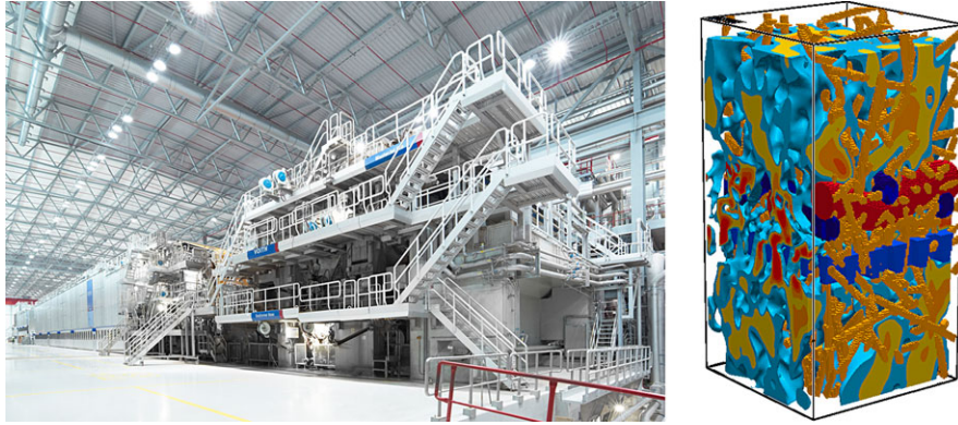
Fig. 6 Left: Press section of a paper machine (Foto: Voith GmbH). Right: Microstructure simulation of a press felt
