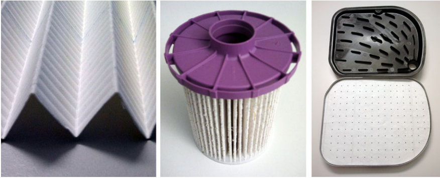
Fig. 1 Left: A pleated filtering medium with corrugation. Center: A pleated cartridge for fuel filtration. Right: Disassembled housing of an automatic transmission oil filter. The filtering medium is perforated and the plastic covering has a supporting rib structure optimized for low flow resistivity
