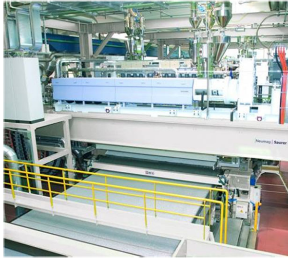
Fig. 11 Spun-fleece process installation with three spinning beams: spunbond–melt-blown–spunbond (Photo: Oerlikon Neumag)
