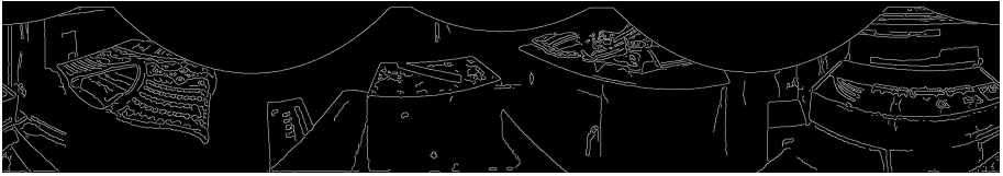
Fig. 6. The Canny edge detection result based on the cylinder panoramic images generated from the low hyperbolic mirror.
