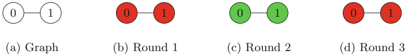
Fig. 7. Example of an infinite loop in SIMT-style parallelism when using one of the optimistic coloring algorithms (Color figure online).
