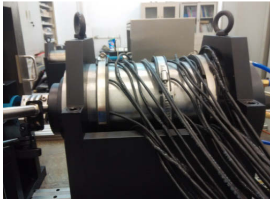
Fig. 4 Thermocouple sensor on motorized spindle
