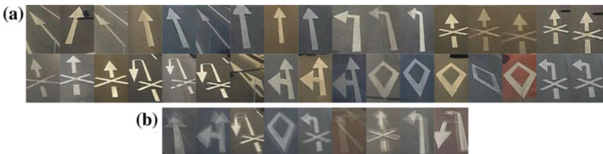
Fig. 6 Sample images for template matching. a Sample images of road surface indicators. b Average images of each road surface indicators
