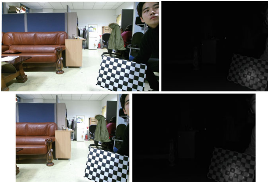
Fig. 3 Above original color and IR images. Below registered color and IR images obtained by the transformation and cropping
