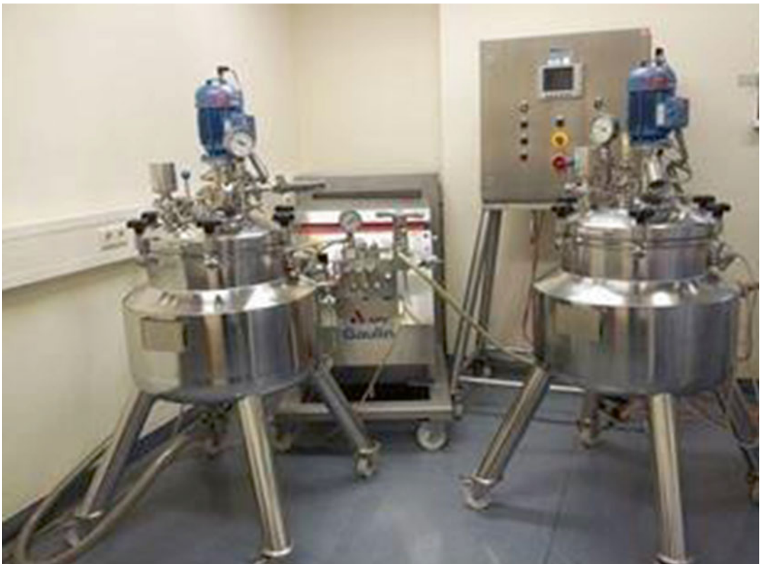
Fig. 11.5 Large-scale production line for lipid nanoparticles – from left to right : feeding container, APV Gaulin 5.5 homogenizer (manufacturer, country) and control unit (both in the back), and product container at the right . Product containers are made of pharma steel and can be
