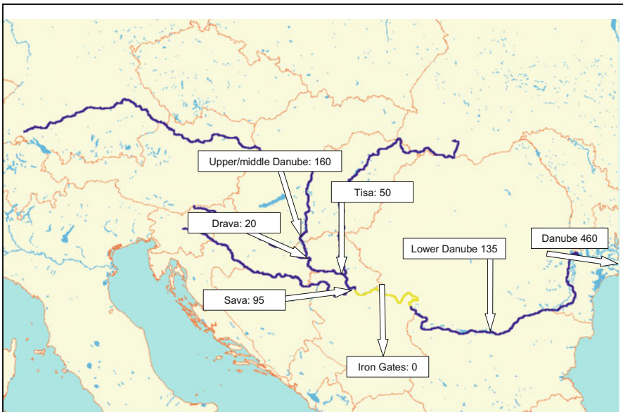
Fig. 6 DIN in-stream loads (kt/year) of the Danube River (based on data from 1997 to 2001)
