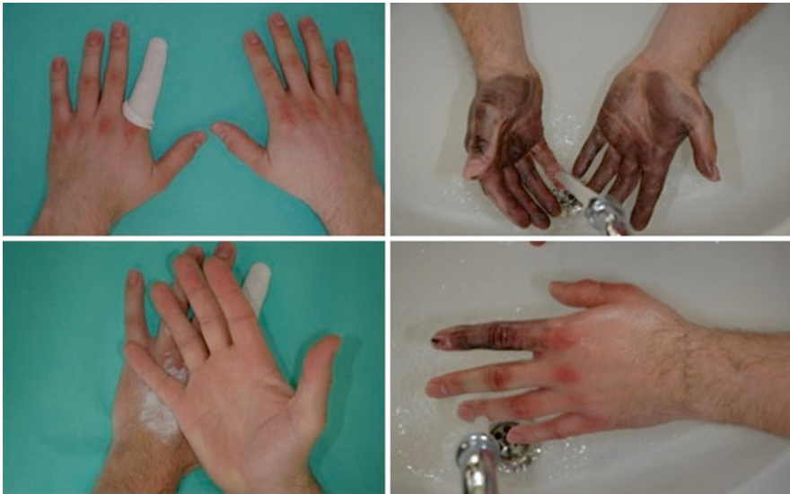
Fig. 24.5 Easier cleaning of the skin after applying barrier cream before work with grease or oil. Experiment to demonstrate this effect: Apply barrier cream (one finger is omitted) and use oily “standard” dirt; the dirt can be rinsed off easily without rubbing or using soap, and only the omitted finger remains dirty
