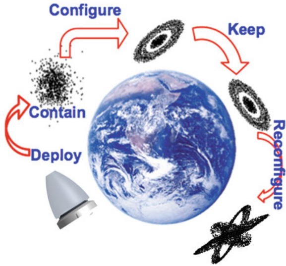
Fig. 2.8 In this example scenario, thousands of spacecraft are deployed in Earth orbit. First they match their periods to ensure that they do not quickly drift apart. Then they configure themselves in order to achieve a desired prescribed pattern. The motion of this pattern is determined by the Earth orbital dynamics
