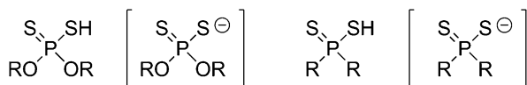
Fig. 2.1 (Left) General structure of dithiophosphoric acids and dithiophosphates. (Right) General structure of dithiophosphinic acids and dithiophosphinates
