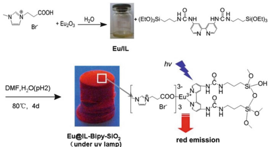
Fig. 7.8 Illustration of the procedure used to obtain the transparent and luminescent ionogel (Reproduced from Ref. [53] by permission of the Royal Society of Chemistry)
