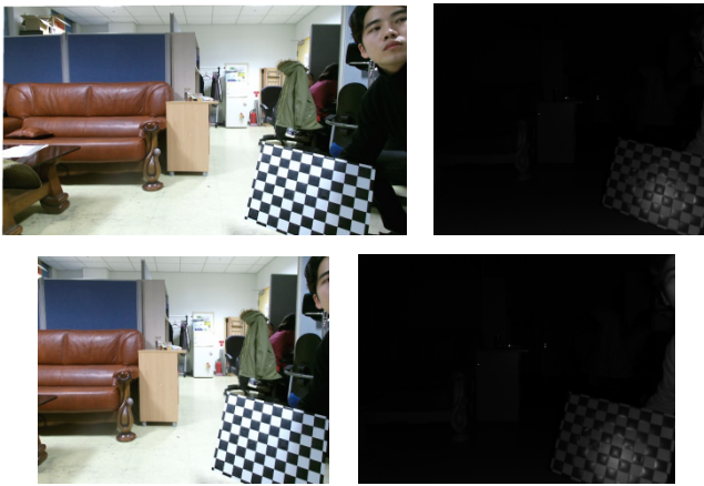
Fig. 3. Above: original color and IR images. Below: registered color and IR images obtained by the transformation and cropping.
