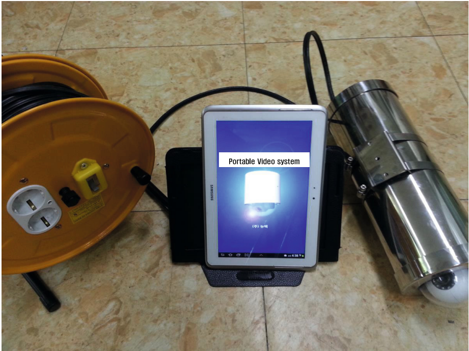
Fig. 6. Developed farm growth monitoring system
