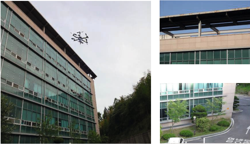
Fig. 4. Recorded images and also hexa-copter used in the experiment
