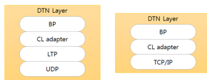
Fig. 5. DTN layer with LTP (left side) and DTN layer with TCP/IP (right side)
