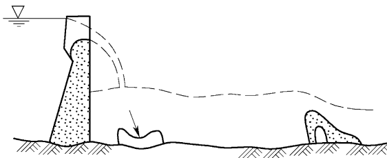
Fig. 8.39 Plunge pool the Calderwood Dam (USA, H = 71 m)
