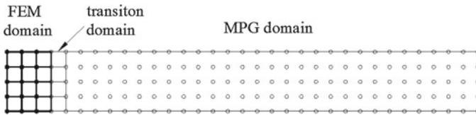
Fig. 5 Discretized model of the cantilever beam
