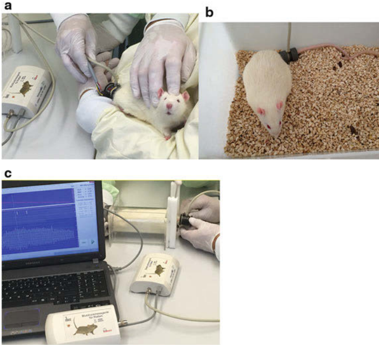
Fig. 9 This figure shows that HDO measurements made in the rat are possible when either minimally restrained (a), freely roaming (b) or while in a tube restrainer (c). Note that the restrainer-derived HDO measurements do not appear stressful and result in measurement of excellent traces, as shown on the monitor (c). Note that freely roaming rats tend to move during recording of the measurements creating possibly too many artefacts for analysis
