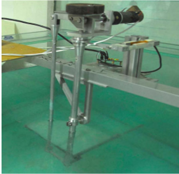
Fig. 5 The bionic pectoral fin imitating manta ray
