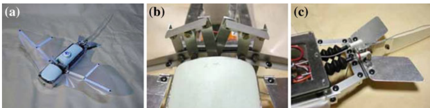
Fig. 7 The first robotic fish propelled by oscillating pectoral fins. a Prototype, b drive mechanism, c tail unit
