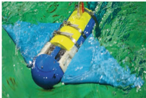
Fig. 10 The bionic fish developed by University of Virginia
