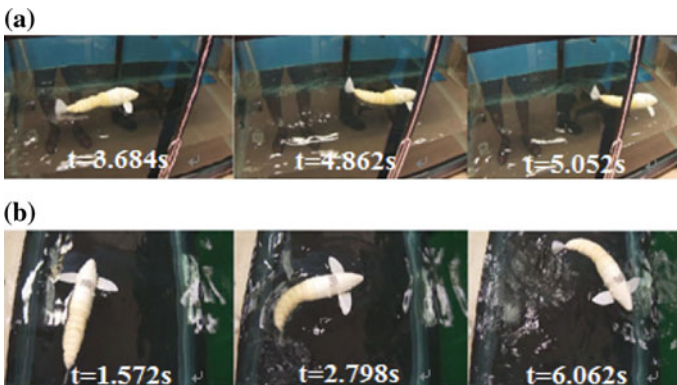
Fig. 23 Swimming with the wire-driven tail alone: a swimming forward; b turning
