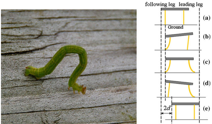
Fig. 7 An inchworm-inspired biomimetic locomotion [35]
