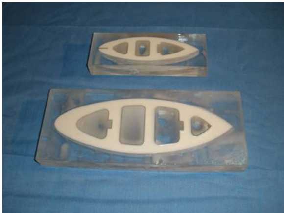
Fig. 41 The mould of chordwise supporting silicon rubber rib
