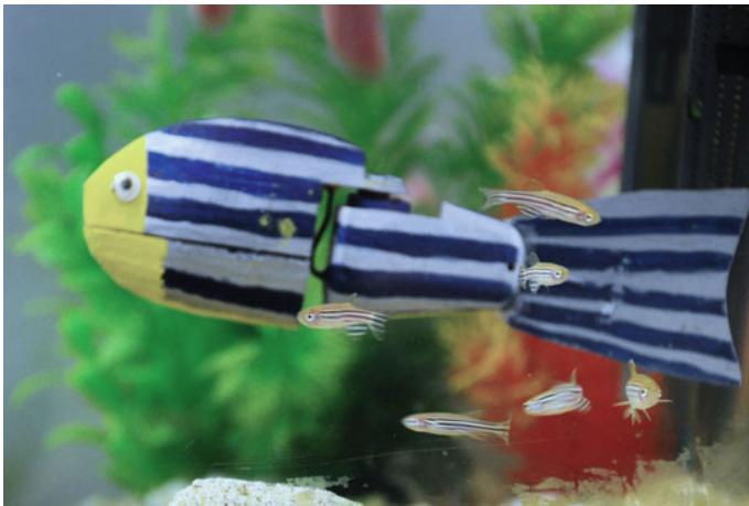
Fig. 1 The robotic fish is designed to match the zebrafish color pattern, aspect ratio, and caudal fin shape. The robot has onboard electronics and motor that allow it to swim autonomously
