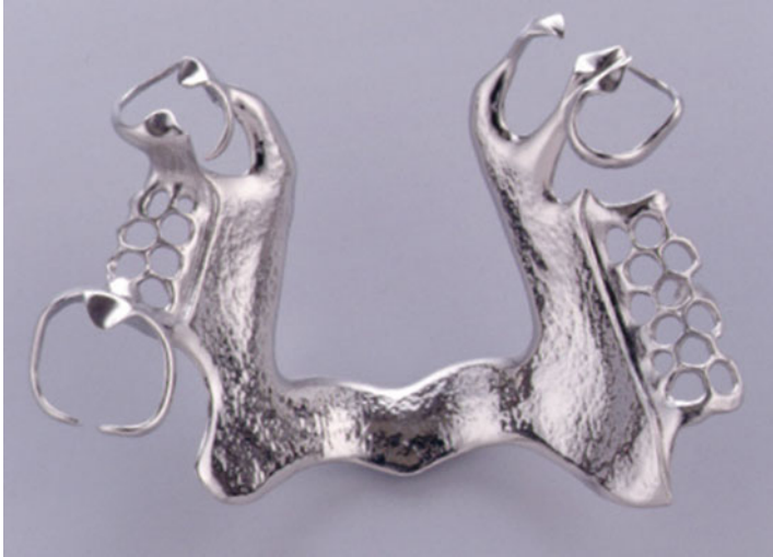
Fig. 12.11 Metal frame of partial denture made from Ti-6Al-7Nb alloy (Reprinted from Ref. [1], Copyright 2010, with permission from the Japan Institute of Metals)
