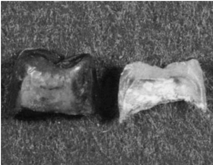
Fig. 12.1 Silver alloy tarnishing (Reprinted from Ref. [1], Copyright 2010, with permission from the Japan Institute of Metals)
