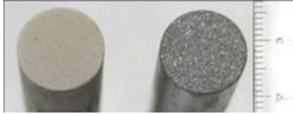
Fig. 7.2 Photograph of surface before bonding ( left : HAp-coated surface, right : blast surface)
