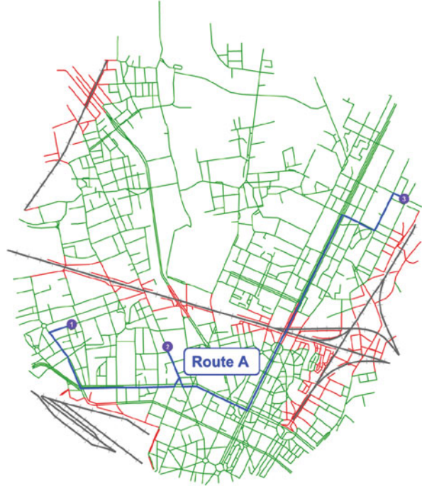
Fig. 14.7 Risk on infrastructures. Darker lines (red colour) correspond to higher risk; lighter lines (green colour) to low risk
