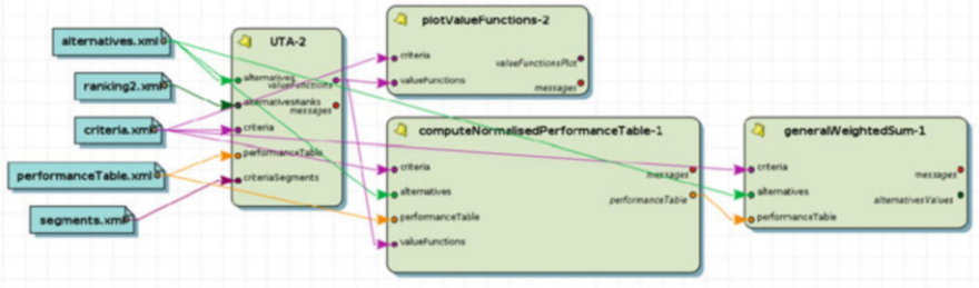
Fig. 21.14 The workflow representing the input data ( left ), the UTA module, the plot module and the normalization module ( center ), as well as the summation module ( right )
