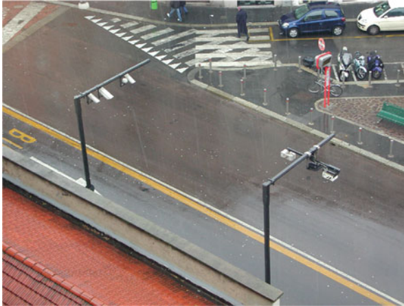
Fig. 14.1 One of the gates equipped with cameras for vehicle plate number recognition
