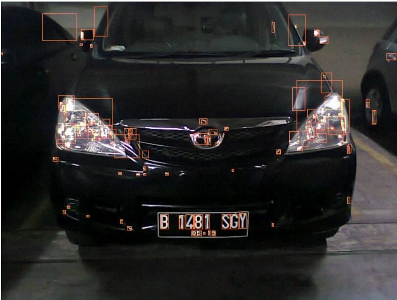
Fig. 4. Segments candidates on original image (marked with orange squares)
