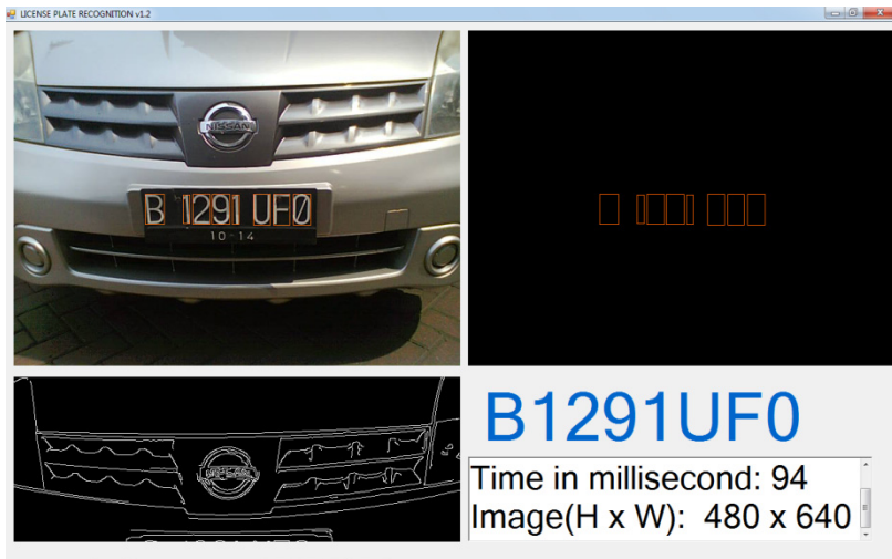
Fig. 10. Application of plate reading at outdoor bright sun light
