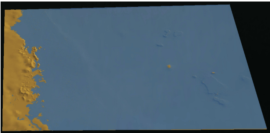
Fig. 2. Simulation result after 5000 seconds of a fixed incoming water flow from the ocean boundary. Flood inundation occurs at the Cairn coastal region.
