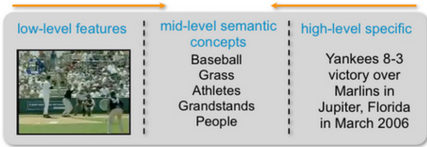
Fig. 2. Semantic gap between machine's extracted information and human's observed information (Source: http://www.research.att.com/projects/Video/VisualSemantics )
