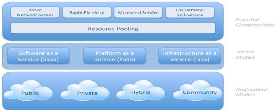
Fig. 1. Visual Model of NIST Definition of Cloud Computing. Source: (CLOUD), IEEE International Conference, pp 516-524).
