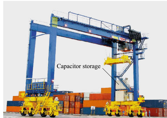
Fig. 16.40 Rubber tired gantry crane that has been hybridized using capacitor energy storage. The repetitive-motion operation of this system makes it ideal for energy harvesting. Typical reported fuel saving is 40% (courtesy of Nippon Chemi-Con Corporation) [16.470]
