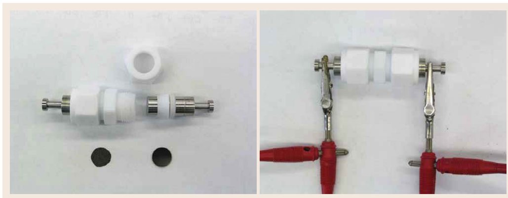
Fig. 17.24 A pair of stainless steel rods act as current collectors in a cell constructed from a Swagelok-type compression union
