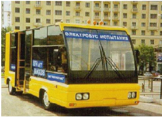
Fig. 16.38 Electric bus powered solely by an electrochemical capacitors. Range is limited to \approx 15 km but charge time is less than 15 min, providing near continuous operation over a circular route (courtesy of ELTON Joint Stock Company)
