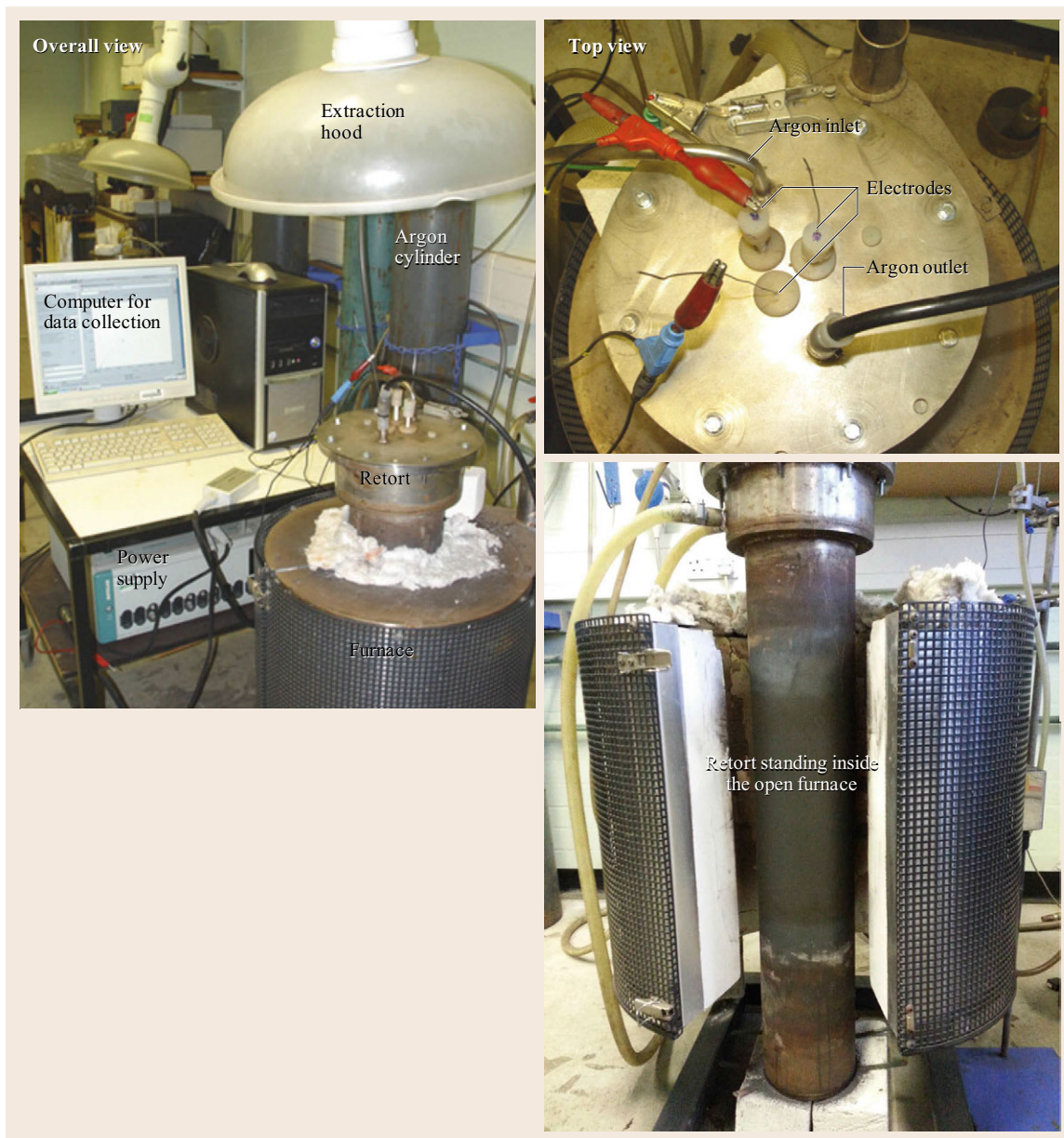
Fig. 25.18 A typical experimental setup of the FFC Cambridge process
