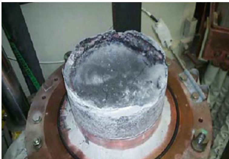
Fig. 25.7 Solidified electrolyte and Ti cathode from the GTT process (after [25.28])
