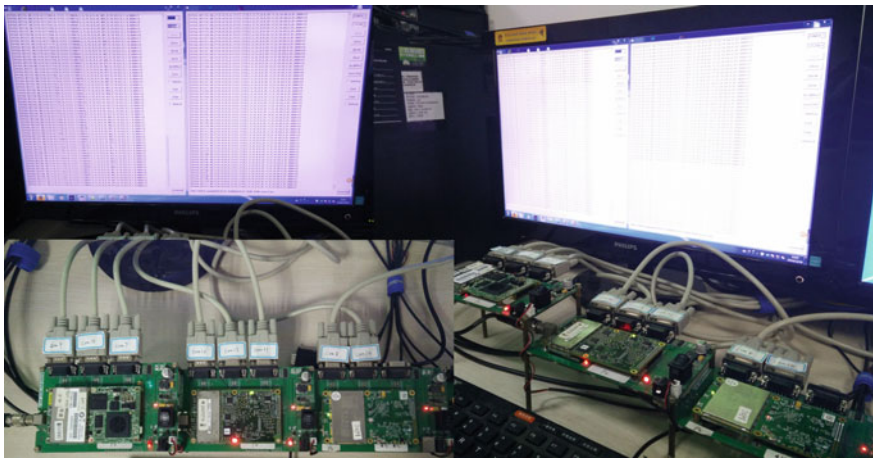
Fig. 70.6 Tests on 0.5-cycle biases of carrier phase between different GNSS OEM boards
