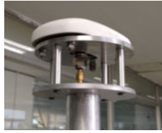
Fig. 53.10 Photograph of the satellite navigation antenna
