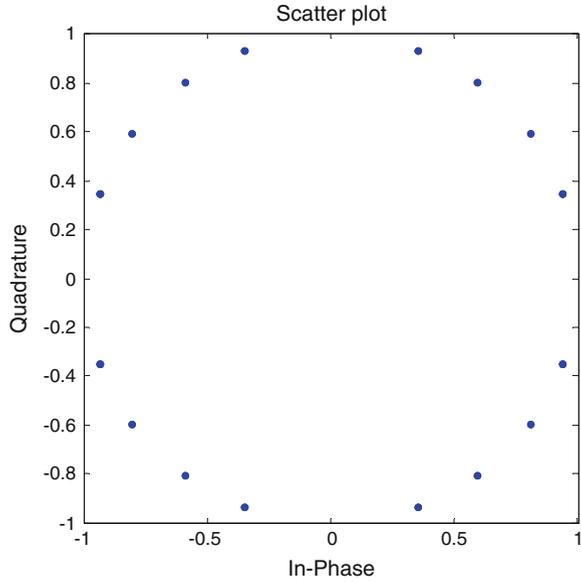
The constellation of GCE-BOC<sub>(1,3)</sub> modulation used in the first multiplexing scheme is shown in Fig. 5.1.
