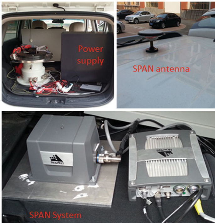
Fig. 58.5 Equipment set-up on the test vehicle
