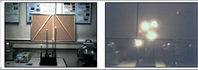
Fig. 4. Four LED lights on the same plane are displayed and used as radioactive sources
