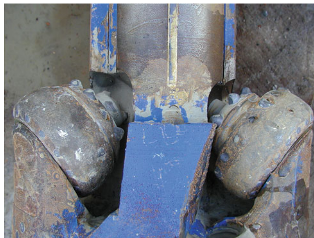
Fig. 7.7 The 6½ in cones of the reaming bit were worn flat
