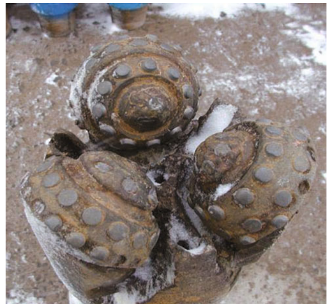
Fig. 7.9 Falling-off of the pilot body of KZ157/244.5-22 bit
