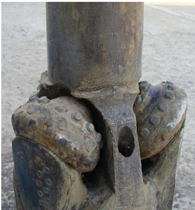
Fig. 7.20 Seriously worn pilot body in MH-2K-21 roundtrip
