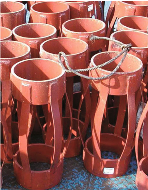
Fig. 10.32 Elastic centralizer for 193.7 mm moving casing
