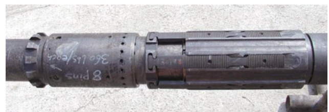
Fig. 10.22 127 mm tail pipe hanger
