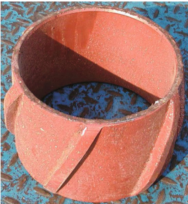
Fig. 10.33 Rigid centralizer for 193.7 mm moving casing
