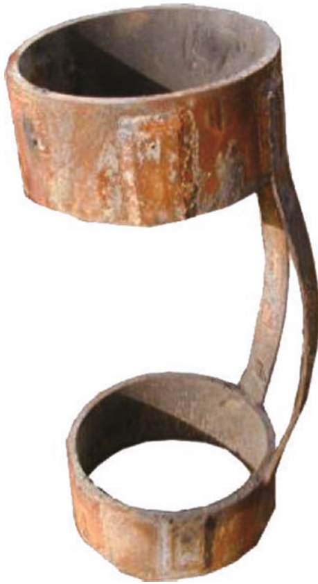
Fig. 10.36 Elastic centralizer with elastic steel strips broken off
