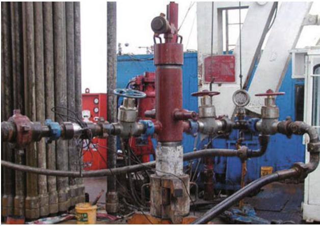
Fig. 10.20 Cement head for 193.7 mm casing cementation
