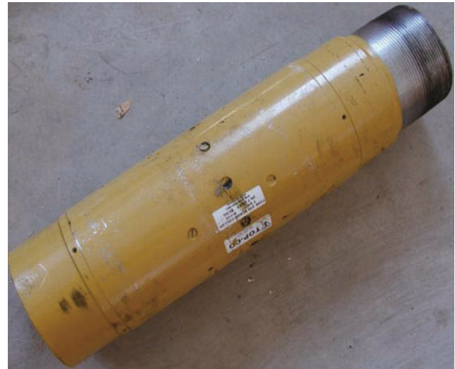
Fig. 10.16 193.7 mm stage collar
