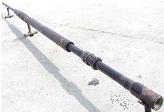
Fig. 10.23 Running-in tool assembly for 127 mm tail pipe
